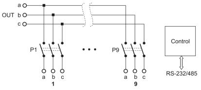
Fig. 2 Block diagram.
