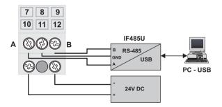
Img. 2.2 Power and RS-485 connections
