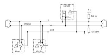
Fig. 2.3 Recommended connection of the RS-485 Modbus-RTU interface
