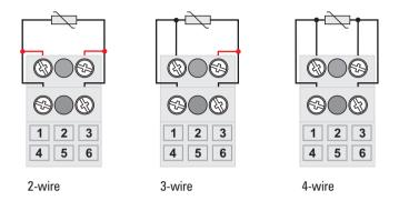
Img. 2.1 Sensor wiring configurations
