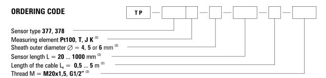
**Example for order:** TP-377Pt100-6-50-1,0-G1/2" Pt100 resistance sensor of outer diameter  $\emptyset = 6$ mm, length L=50mm,
