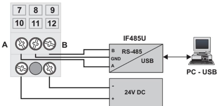
Img. 2.2 Power and RS-485 connections
