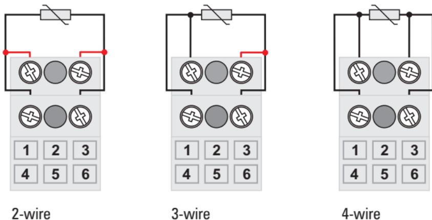
Img. 2.1 Sensor wiring configurations
