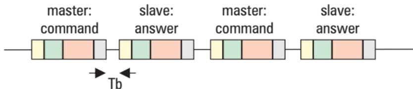
Tb - interruption in access to the bus:  $\min 3.5 \cdot$  transmission time of a single byte (11 bits)
